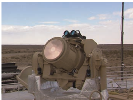
The Tactical High Energy Laser (THEL) pointer-tracker which follows the target and points the laser
