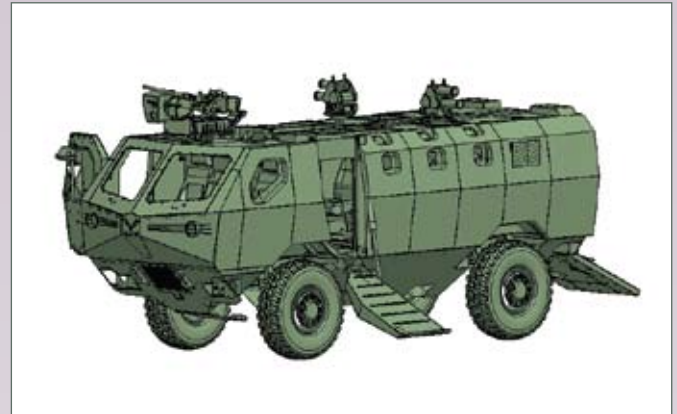
The IMI Wildcat was developed from a commercial truck chassis. It has near identical performance and capability characteristics to the US M-1127 Stryker, and includes an active protection system [IMI]
