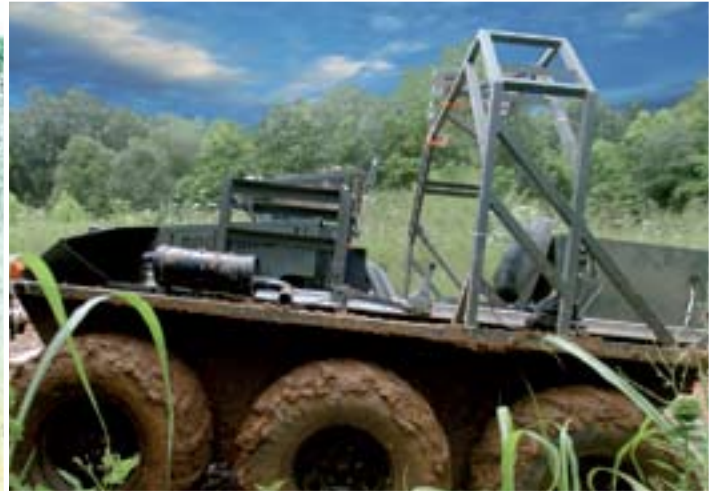
An unmanned SMSS breezes along a country path in supervised autonomy mode [Lockheed-Martin]
