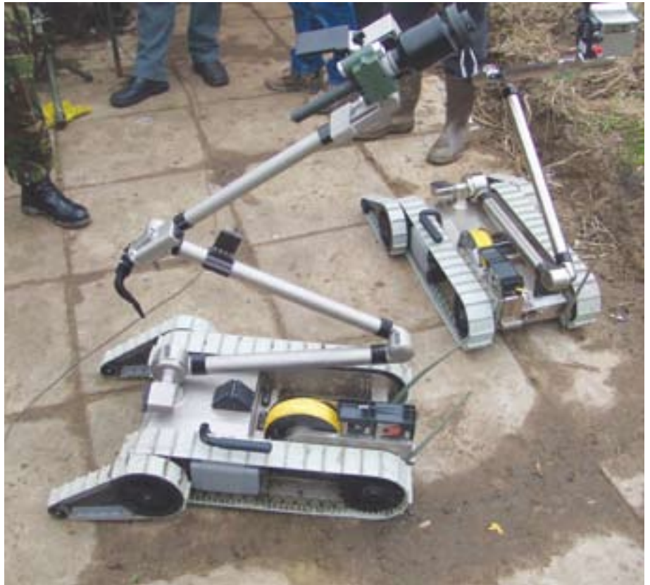
Two Packbots on trial at the Army School of Ammunition [Army School of Ammunition]
