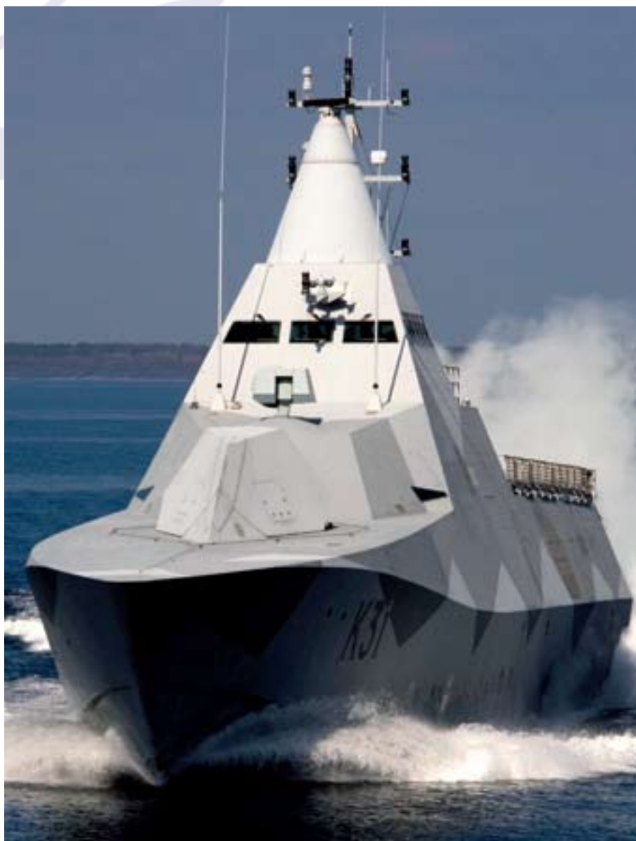
Stealth is a very important part of the Visby corvette concept [Peter Nilsson, Kockums AB]
