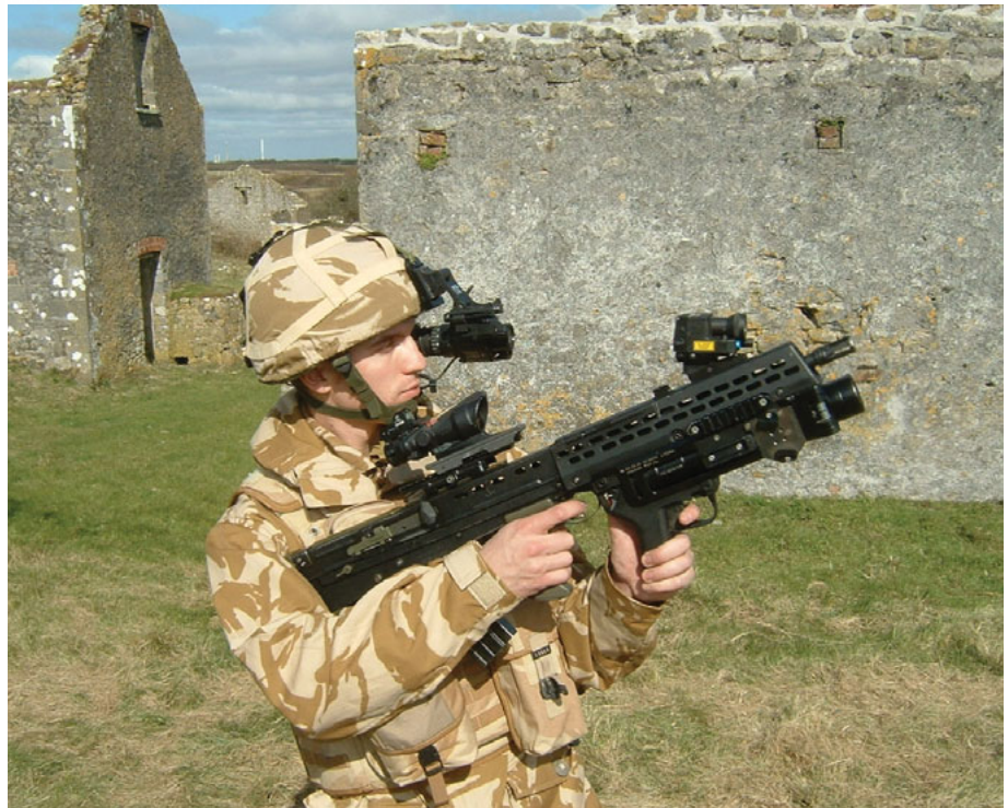
A soldier wearing a Head Mounted Night Vision System (HMNV), and using a SA80A2 rifle fitted with an ACOG battle sight and a 40 mm underslung grenade launcher (UGL)
