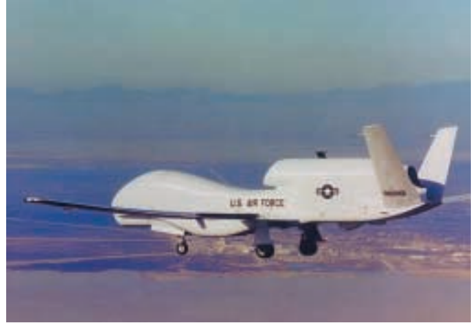
The Northrop Grumman Global Hawk is a high-altitude, long-endurance unmanned aerial reconnaissance system.
